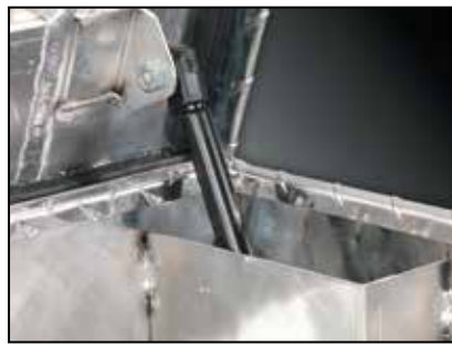
The cover support housing protects the gas springs.
