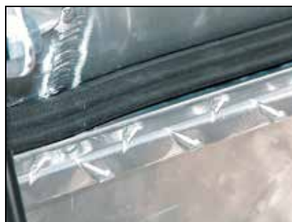
Full weather stripping keeps dust and moisture out.
